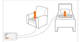
Programmable absence delays from 0.5 secs to 30 mins. Start/ Finish timings available on Notifier / compatible DAU.
