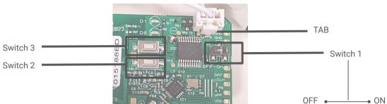
Firstly, unpack the unit and separate the sensor from the mounting plates. Turn Switch 1 on the PCB into the ON position (see picture). The LEDs will flash rapidly red and orange.
